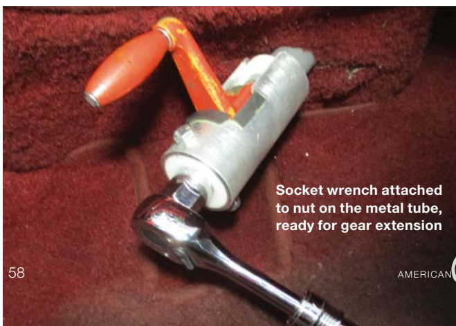
Extension assist tool slipped around the extended hand crank
