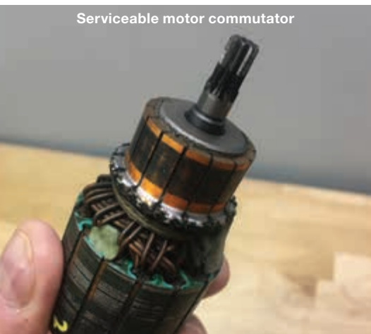
This commutator needs to be turned.
