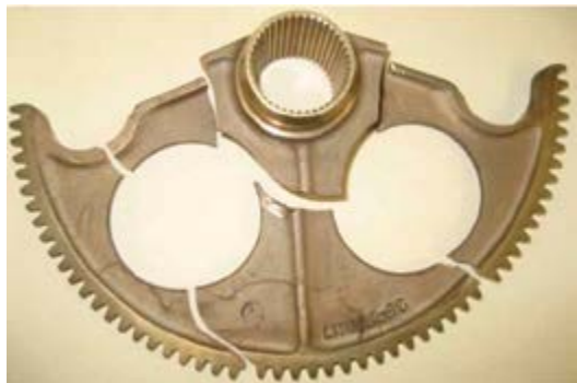
Figure 4: A sector gear that shattered as a result of mis-rigged limit switches and repeated powered contact with the internal stop
